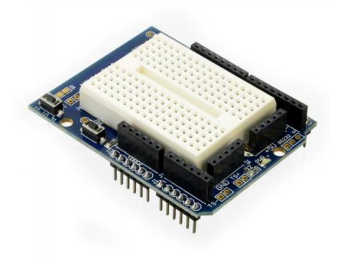
Shields are designed to sit on top of an Arduino board, simplifying its interface and making it easier to prototype and work within a small space with multiple wires.
