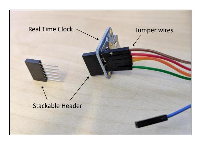
The Real Time Clock has a through hole connection, which can make it difficult to secure Jumper Wires.
