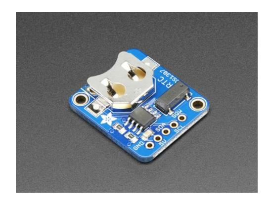
When a weather station logs a recoding, the Real Time Clock will ensure it logs at the correct time. It requires a battery (not included) to maintain the correct time when power is lost to the Arduino.
