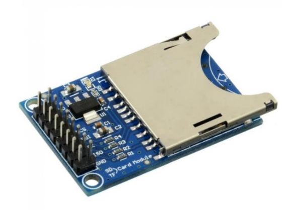
The SD Card Module allows for the Arduino to log the weather recordings to a csv file.
